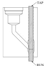
When both conductors are smaller than 1/0: place end of lower cable to <u>bottom</u> of tap hole, then butt upper cable against lower cable
