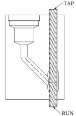
Place end of lower cable to center of tap hole, then butt upper cable against lower cable
